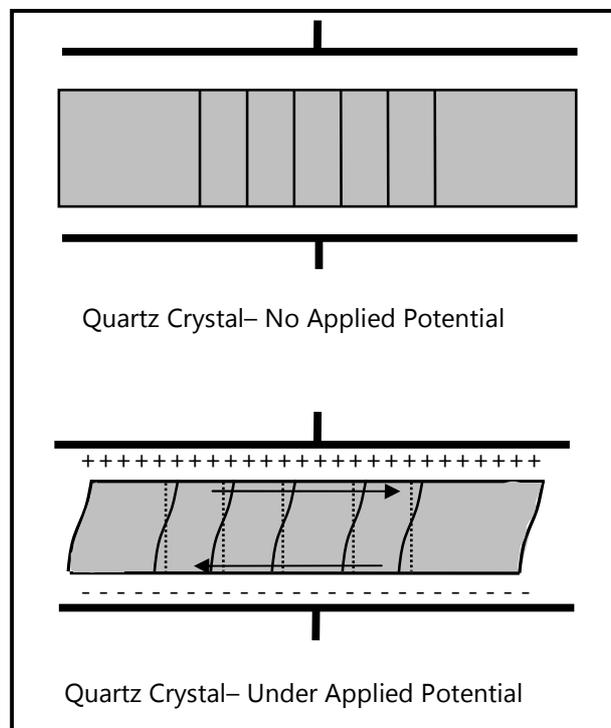
**Figure 1. Graphical Representation of Thickness Shear Deformation.**
