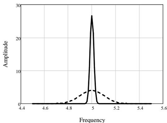
**Figure 2. Comparison of High Q and Low Q.**
