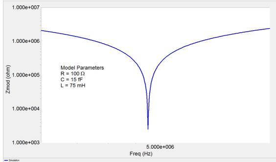
**Figure 5. Impedance Spectrum for a Series RLC Circuit.**
