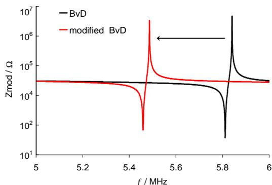
**Figure 9. Comparison of BvD and Modified BvD Models.**
