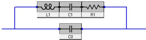
**Figure 6. Butterworth – van Dyke Equivalent Circuit Model.**
