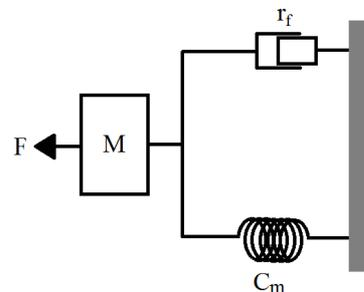
**Figure 3. Quartz Crystal Microbalance Equivalent Mechanical Model.**
