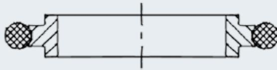
Centering ring with elastomer o-ring (ISO-KF)
